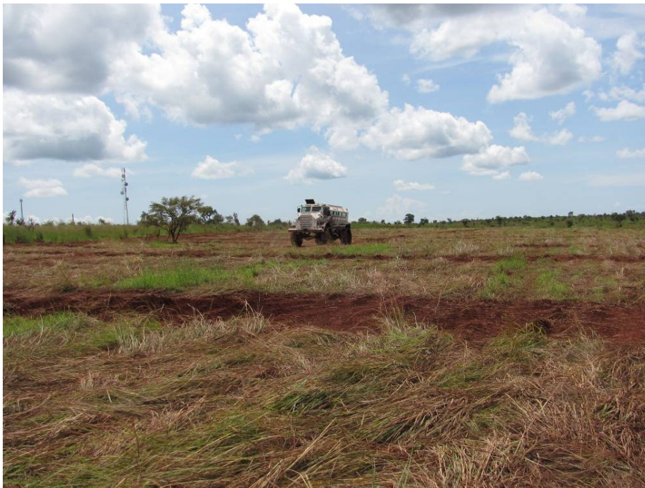
Pict. 5. Mine Protected Vehicle being used with steel wheels for Technical Survey in Angola
