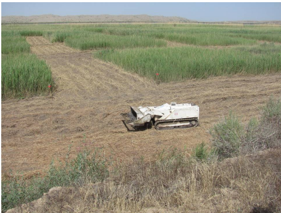
Pict. 2. Medium flail used for vegetation cutting, ground preparation and possibly mine detonation in Tajikistan.
