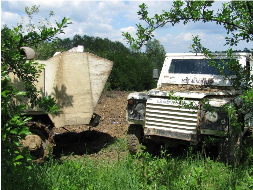
Pict. 3. MPV used to drive remotely a medium tiller from close in Bosnia
