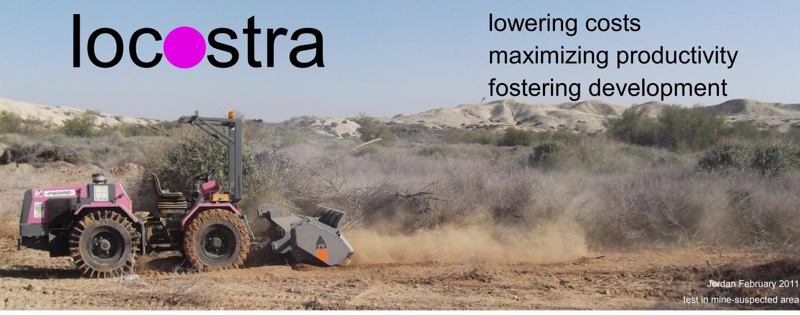
the first machine designed for technical survey, area preparation and agriculture
