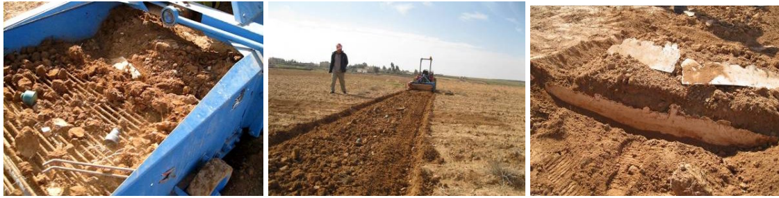
Fig.2. Performance test of LOCOSTRA equipped with ground processing tool (potato digger).
