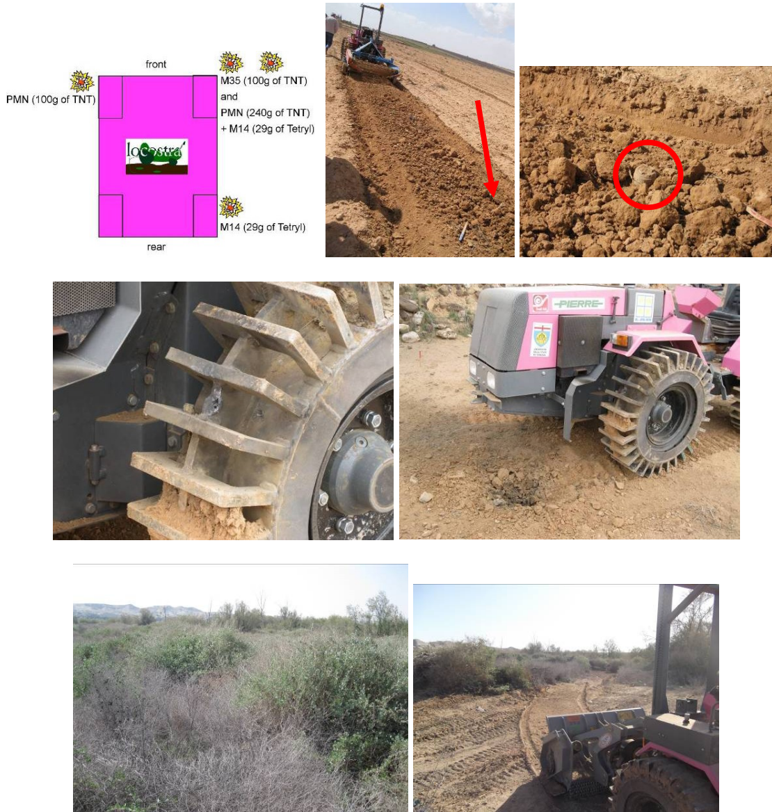
Fig.3. Explosions occurred under LOCOSTRA, an M14 mine removed and processed by the GPT without explosion, the worst damage caused to blast resistant wheels (very light) after a PMN explosion, medium vegetation before and after clearance.
