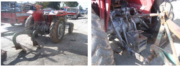
Fig. 11. Small Jordanian tractor and its three point linkage.
