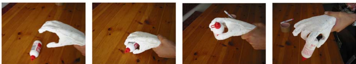
Figure 7 – Prototype of underactuated hand, with mechanics and actuation integrated in an elastomeric structural matrix.
