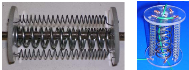
Figure 4 – Robotic modules for steering and peristaltic trust.
