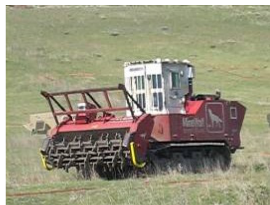
Fig. 2.5. The two mostly used mechanical demining technologies: flail and tiller.
