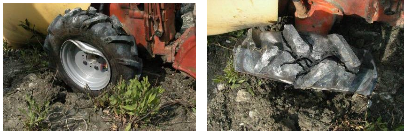
Fig.5.27. Wheel filled in with GoFill after first explosion, seen from the side, after 180° rotation and from the top.
