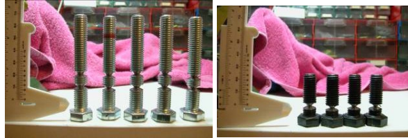
Fig.5.23. Screws with double and single cut to be tested as alternative breakable connection.
