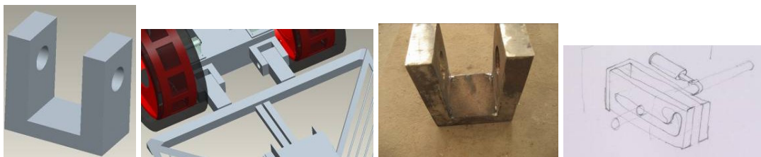
Fig.6.29. Hitch module final model, assembly on the model and prototype.
