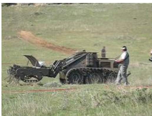
Fig. 2.5. The two mostly used mechanical demining technologies: flail and tiller.
