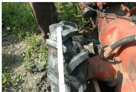
Fig.5.36. Tyre after second test, seen from the top, after 180° rotation.
