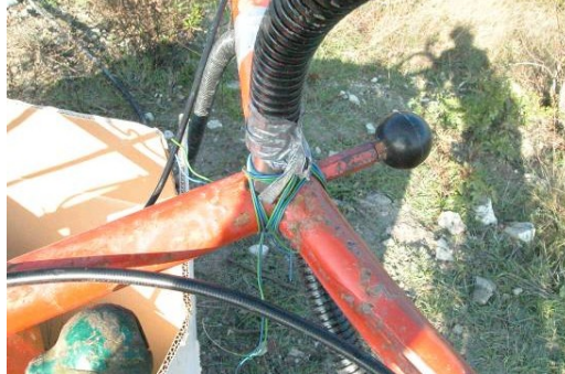
Fig.4.33. Arrangement of the accelerometer on the handle bar.
