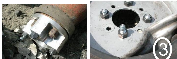
Fig.5.43. Screws with double cut broken after third test.
