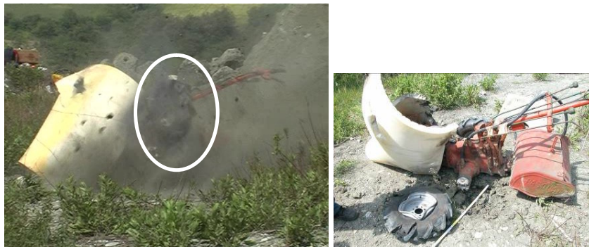
Fig.5.59. Picture of power tiller during fourth test, taken from the video recorded and powertiller after test.
