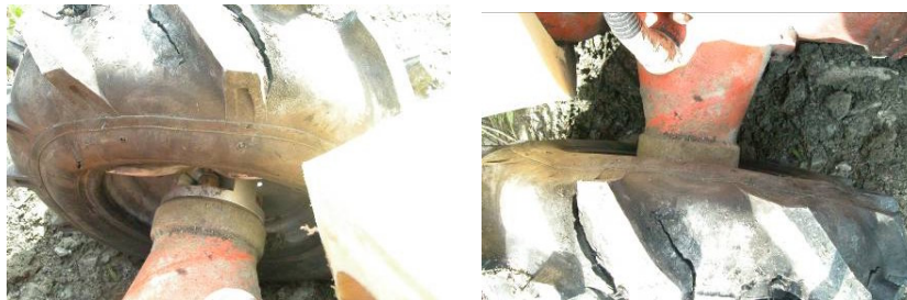
Fig.5.28. Wheel filled in with GoFill after first explosion, seen from the internal side, after 180° rotation.
