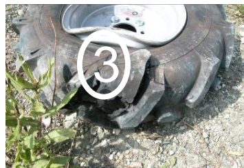
Fig.5.42. Tire after third test, dropped off on the ground.
