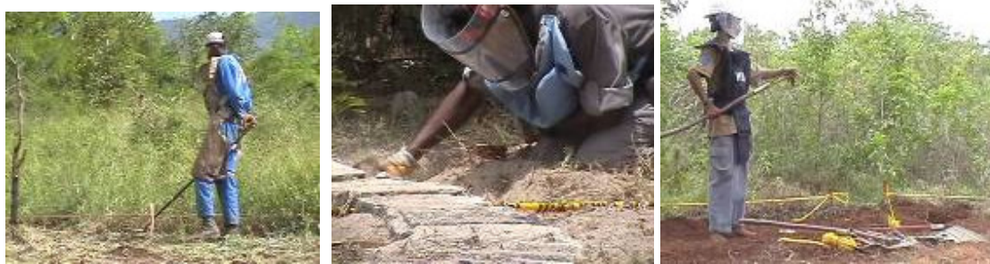
Fig. 2.4. Deminers equipped with different tools: metal detector (ADP, Mozambique), trowel (FSD, Sri Lanka), and rake (MAG Sri Lanka).
