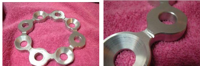
Fig.5.24. Breakable ring with all bridges cut, to be tested.
