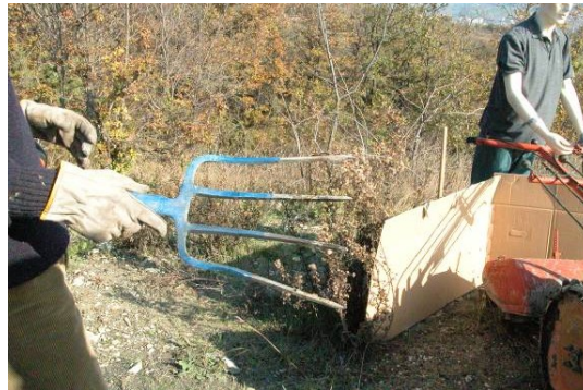
Fig.4.32. Damages on the rake after the fourth test.
