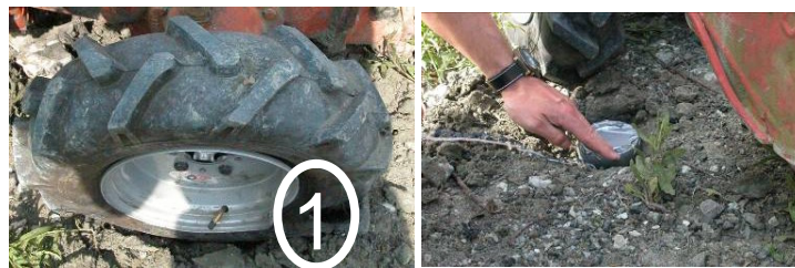
Fig.5.34. Wheel filled in with GoFill in position for the second test and mine placement.
