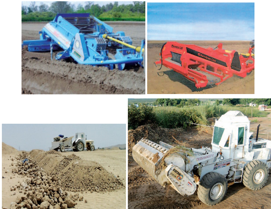
Fig.2.9. From the top left: Pearson Sifter, Armtrac Sifter, KZ Sifter and HEC Rotar (Source: Mechanical Demining Equipment Catalogue 2006).
