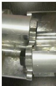
Fig.5.22. Plastic deformations of the breakable ring after the pre-test.
