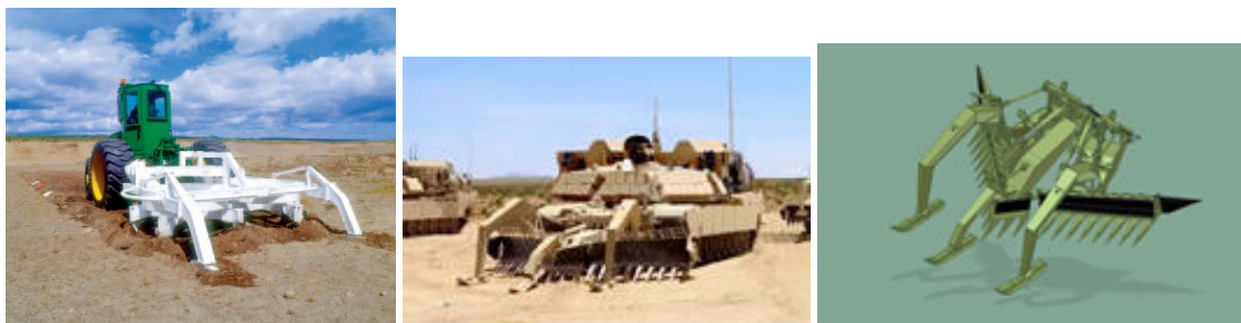
Fig.2.10. From left to right: Pearson Mine Comb (Source: Mechanical Demining Equipment Catalogue 2006); Pearson Mine plough attached and in details (Source: http://www.pearson-eng.com ).
