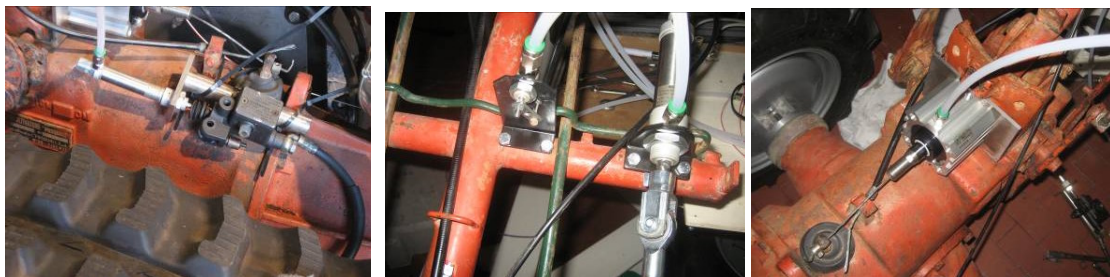
Fig.8.7. Valve bay (provisional box) and fixtures for brakes, acceleration, differential and clutch.
