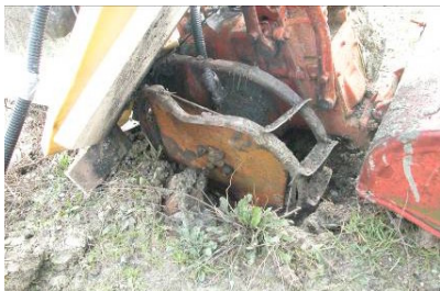
Fig.4.29. Damages on the dummy, power tiller chassis and left wheel after the third test.
