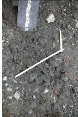
Fig.4.20. Test n°1: crater of the explosion (each segment of the metre is 20 cm long).
