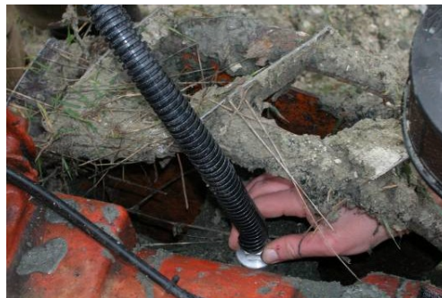
Fig.4.21. Accelerometer on the wheel axis.
