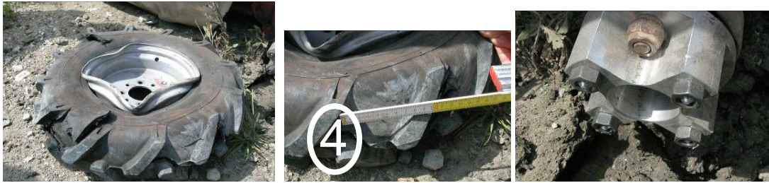
Fig.5.60. Tyre after fourth test, dropped off on the ground and screws with single cut broken after forth test.
