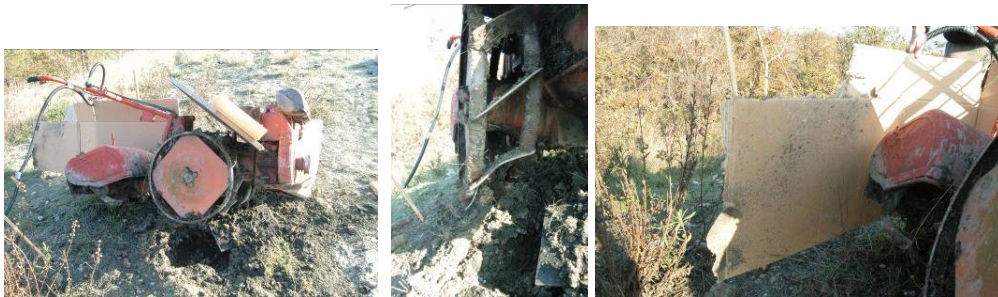
Fig.4.34. Damages on the power tiller right wheel and cardboard after fifth test.
