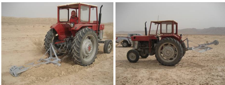
Fig. 7.16. Testing system (tractor driven backwards plus three point frame for supporting the tool) and use of chain.
