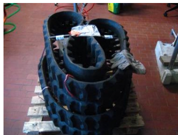
Fig.6.16. Tracks, 230x72x47, kindly provided for free by Minitop.
