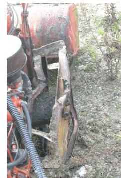
Fig.4.29. Damages on the dummy, power tiller chassis and left wheel after the third test.
