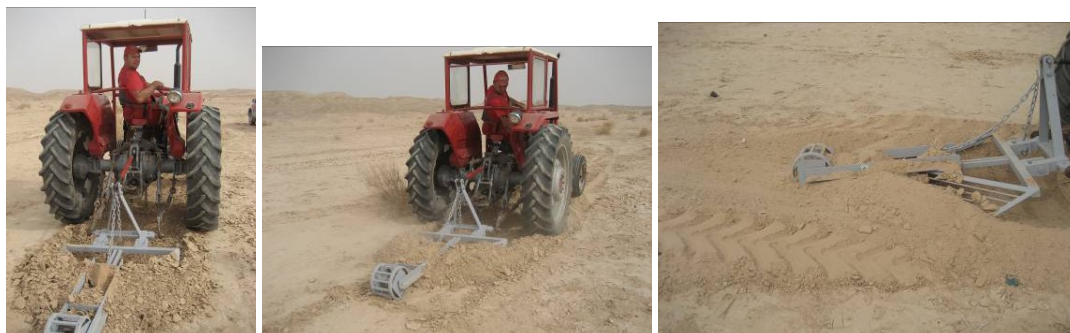
Fig. 7.18. Soil processed by the ground processing tool. A landmine pushed to the side can be seen (green).
