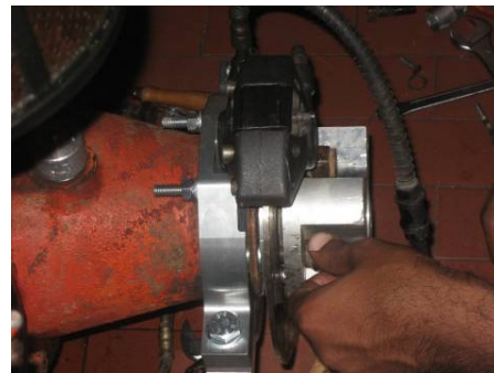
Fig.6.12.a.Brake fixtures conceptual design and assembly.
