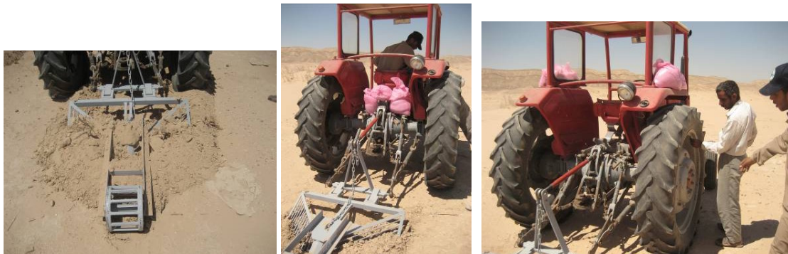
Fig. 7.19. Soil processed by the ground processing tool moved right under tractor wheels. Adding weight on wheel axis (pink bags) and decreasing tire pressure.
