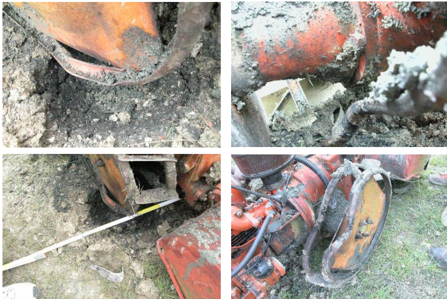
Fig.4.23. Damages on the power tiller chassis and left wheel after the second test.
