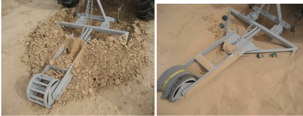
Fig. 7.20. Soil processed built up on the tool and front wheel sinking in pure sand.
