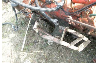
Fig.4.29. Damages on the dummy, power tiller chassis and left wheel after the third test.
