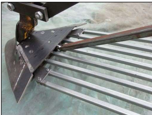
Figure 3: Sweep with cover plate which protects and provides mounting for the sieve
