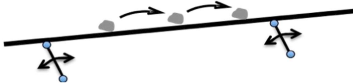
Figure 5: Action of vibratory conveyor
