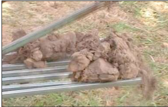
Figure 9: Soil manually placed on screen being conveyed and sieved
