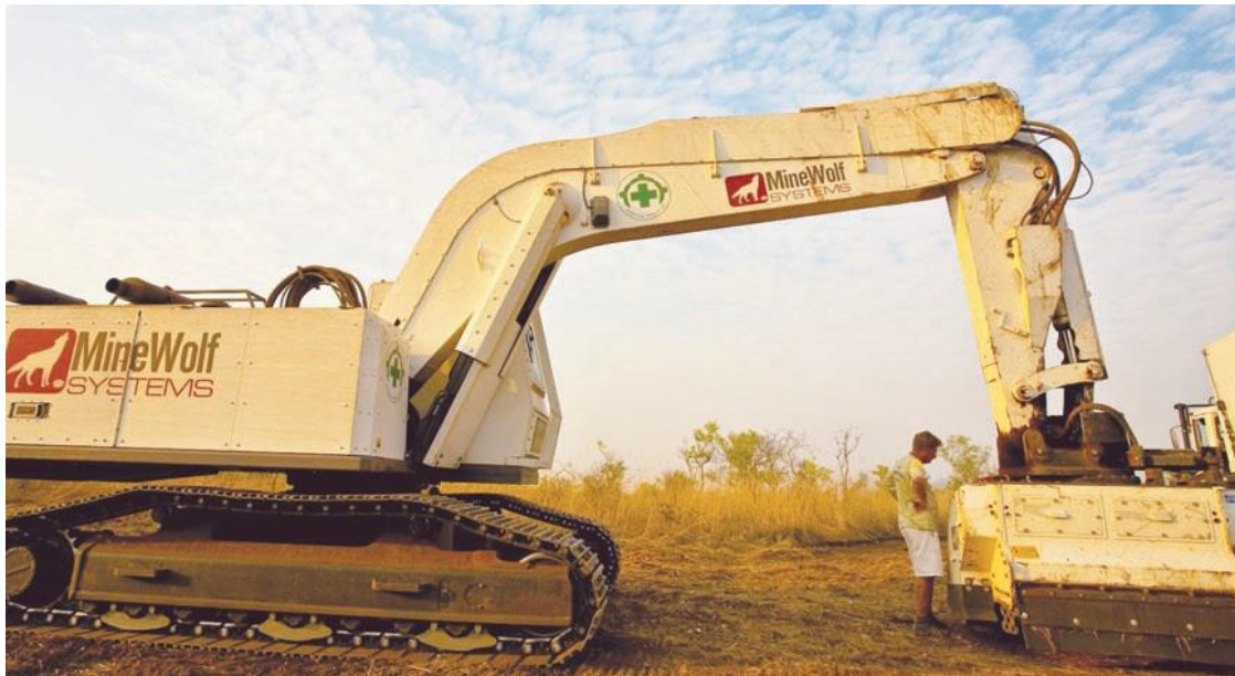
Fig. 1.3 1: The MineWolf Bagger, a machine for ground preparation.
