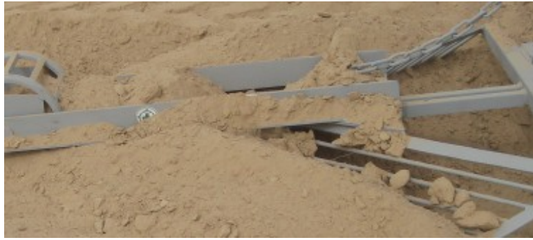
Fig. 2.2 2: The Disarmadillo ground processing tools immersed into the soil.
