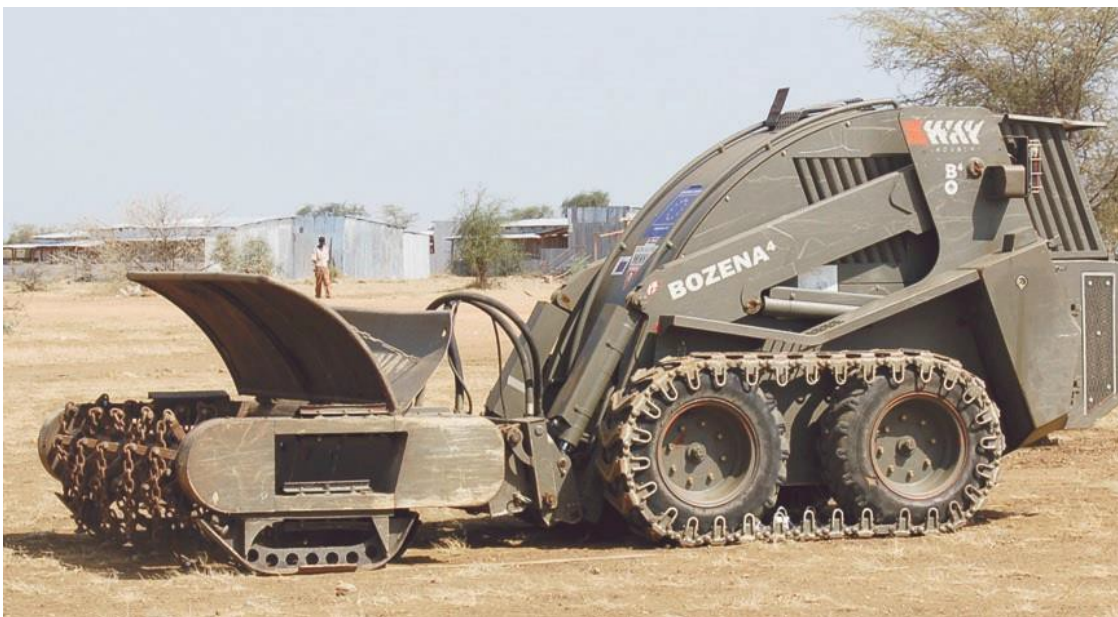
Fig. 1.3 2: The Bozena 4, a machine designed to detonate hazards.
