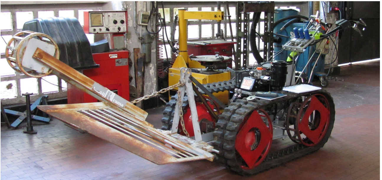
Fig. 2.3 2: Disarmadillo at the beginning of my work. Notice the ground processing tool attached to the front of the frame.
